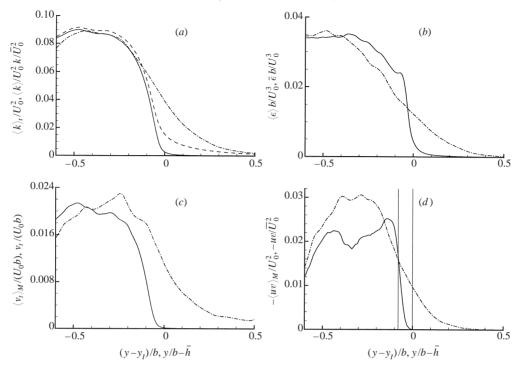
FIGURE 18. One-point statistics based on Eulerian ( $-\cdot-$ ) and conditional averaging, unforced wake. (a) Kinetic energy. ----,  $\langle k \rangle$ ; ———, 'purely turbulent'  $\langle k \rangle_t$ . (b) Dissipation rate. (c) Turbulent viscosity. (d) Shear stress; interface position shown by vertical lines.
