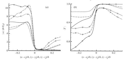
FIGURE 6. Effect of surface orientation on conditional averages of (a) vorticity magnitude and (b) passive scalar in the forced (with circles) and unforced (plain) wakes. Orientation: ...., downstream; —, vertically; — · —, spanwise.
