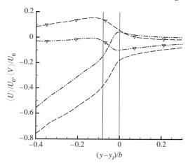
FIGURE 12. Conditional velocities  $\langle U \rangle$  (plain) and  $\langle V \rangle$  (with symbols) for upstream-leaning (----) and downstream-leaning (----) surfaces. Interface position is shown by vertical lines.
