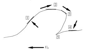
FIGURE 13. Notional arrangement of detected surfaces. Arrows show corresponding typical interface velocities  $(\langle U \rangle, \langle V \rangle)$  relative to free stream. 1, upstream-leaning; 2, outer group; 3, downstream-leaning; 4, inner group. A re-entrant zone is also indicated (5).
