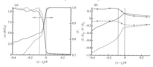
FIGURE 11. Effect of separating interfaces into three groups by height above centreplane, forced wake: —, outer group; —, inner group. (a) Conditional vorticity and scalar. (b) Conditional velocities  $\langle U \rangle$  (plain) and  $\langle V \rangle$  (with symbols). Vertical lines show interface position.
