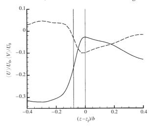
FIGURE 9. Conditional velocities for spanwise-facing interfaces, unforced.
