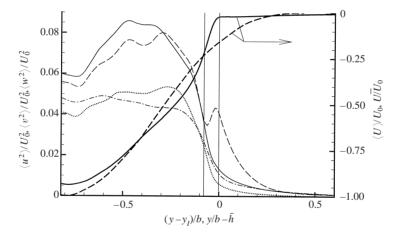
FIGURE 8. Conditional velocity variances relative to conditional means for vertically facing interfaces: —, streamwise; — • —, transverse; · · · · , spanwise. Also shown: conditional (bold solid) and conventional (bold dashed) mean streamwise velocity, and conditional streamwise variance relative to the conventional mean (———). Vertical lines show interface position. The abscissa for  $\bar{U}/U_0$  is  $y/b-\bar{h}$ .
