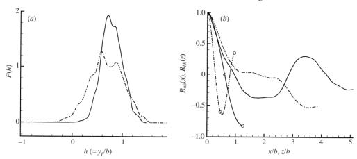
FIGURE 4. Statistics of vorticity surface heights in the unforced (---) and forced (---) wakes. (a) Probability density functions; (b) streamwise (plain) and spanwise (marked with circles) autocorrelations.
