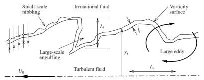
FIGURE 1. The intermittent zone.  $L_I$ ,  $\ell_I$ ,  $y_I$  and  $L_x$  are sketched roughly to scale. Vertical lines on the left typify data selected for y-direction conditional averaging relative to detection points ( $\bigcirc$ ) on the vorticity surface; data at a particular displacement  $y-y_I$  from the surface, e.g.  $\times$ , are averaged to form one point in the conditional average of any quantity, e.g.  $\langle U \rangle (y-y_I)$ .
