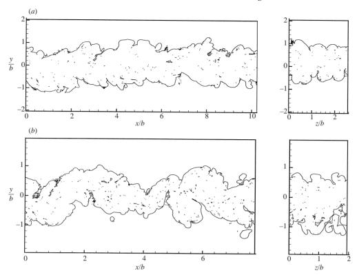
FIGURE 2. Contours of vorticity modulus  $\omega$  in (x, y)- and (z, y)-planes at the levels used for detection of vorticity surfaces. (a) Unforced wake,  $\omega = 0.7U_0/b$ ; (b) weakly forced wake,  $\omega = 1.2U_0/b$ .
