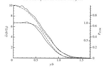
FIGURE 5. Cumulative probability of interface height (--) compared to mean vorticity magnitude (----) in the forced (upper curves) and unforced (lower curves) wakes. The two  $P_{\text{CUM}}$  axes are scaled so that the respective curves match at the centreplane.
